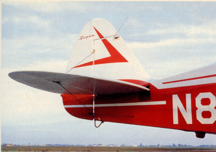
Our Tri-Pacer's wire-braced tail shows off the characteristic 1950s Piper "swoosh," a styling element that we expect to reappear on the final item.
